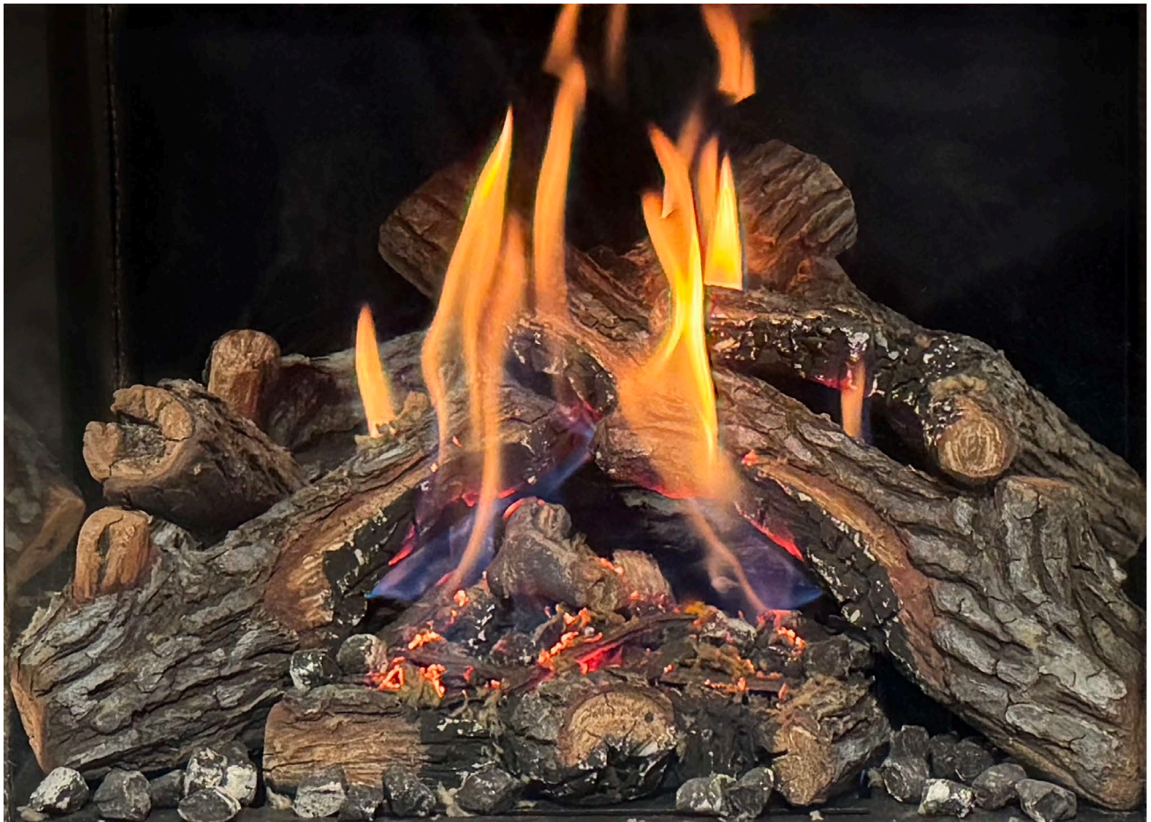
Figure 5-2 Burner Flame Heights: This image provides a visual reference for the burner flames burning at maximum height after the burners have been operating for 30 minutes or longer. A normal rear flame will be 1 to 2 inches above the rear log top edge. This, however, is dependent on the gas type, air shutter opening setting and vent system configuration. Actual flame heights can be slightly higher or lower when compared to this reference image.
